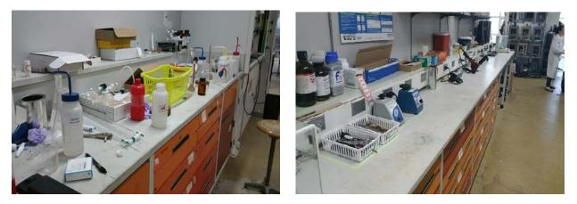
Before and after the 5S standard: frequently used tools are labeled and have outlined locations; excessive supplies and unused equipment reduced; drawers and storage labeled and sorted.
